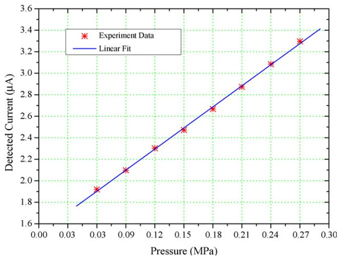
Fig. 7. Acoustic pressure dependence of FBG hydrophone unit.
