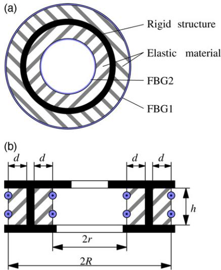
Fig. 2. Hydrophone section view. (a) Cross-section; (b) longitudinal section.
