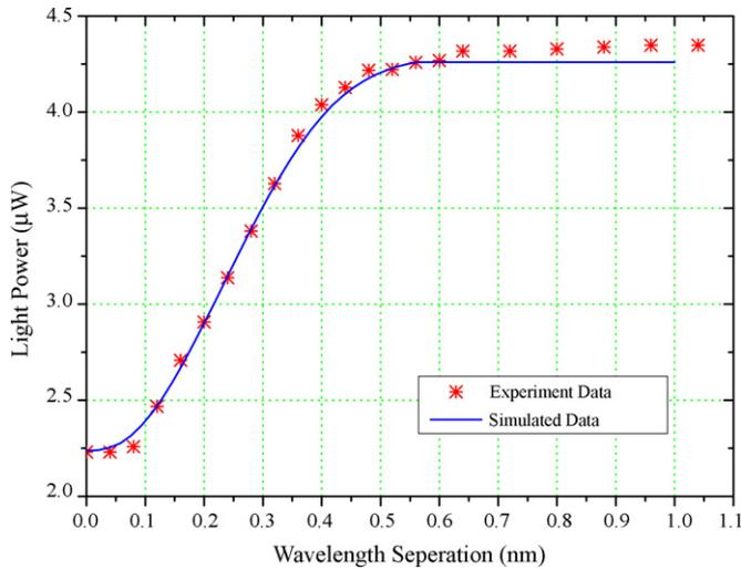
Fig. 6. The relationship between the detected light power and the total wavelength shift of two FBGs.
