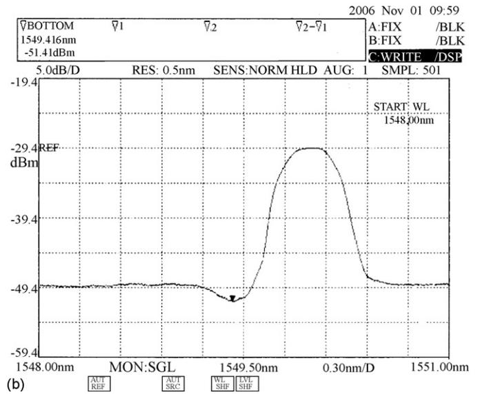
Fig. 8. The received spectrum transforms when pressure varied from low to high. (a) Received spectrum in low pressure. (b) Received spectrum in high pressure.
