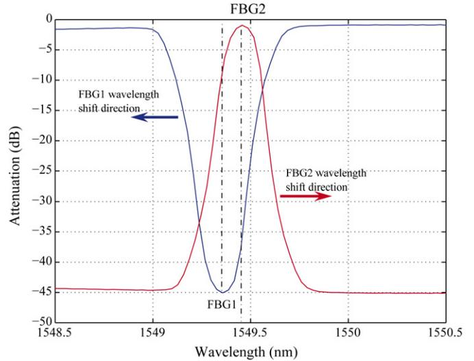
Fig. 5. Self-demodulation demonstration.
