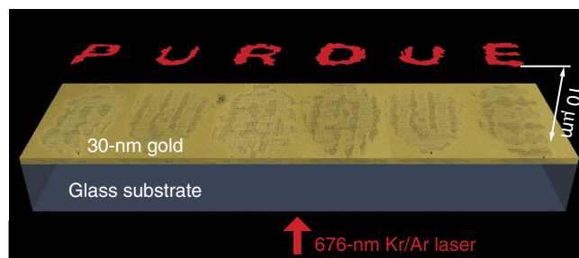
Figure 3 | Holographic images produced by the experimental metasurface holograms. The image is of the word 'PURDUE'. The sample is illuminated by a Kr/Ar laser at 676 nm from the glass substrate side. The images are obtained experimentally at a plane 10 \mu\text{m} above the metasurface hologram. The patterns on the gold film are the FE SEM images of the fabricated samples.
