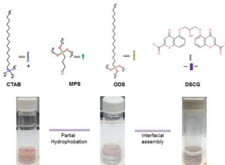
Figure S2. Graphic illustration of surface molecular structures and assembly process during the synthesis of symmetry-breaking gold nanorod dimers. The surface molecules are: cetyltrimethylammonium bromide (CTAB), mercaptopropyltrimethoxysilane (MPS), octadecyltrimethoxysilane (ODS) and disodium chromoglycate (DSCG). The electrostatic interaction is between CTAB (positive charged) and DSCG (negative charged).
